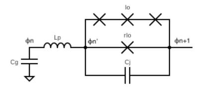
Figure 1: SNAIL TWPA circuit with parasitic inductance.
